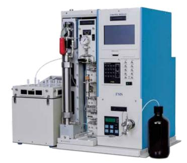
A single module PLE sending oil from 2 ounces of natural product extracted directly to a SuperVap<sup>®</sup> Concentrator. Capable of processing 4 lbs. in 8 hrs.
