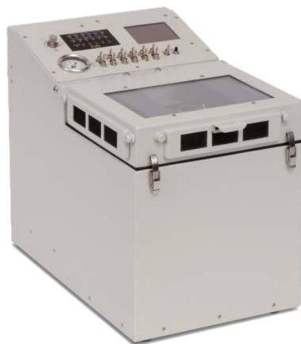
The SuperVap™ Concentrator automatically brings the extract to final volume in an autosampler vial, ready for final analysis. Automatic time-based or endpoint detection shuts off nitrogen for each vessel.
