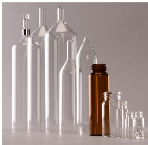
Concentration / evaporation vessels in 500 \mu L and 1 mL, direct to a GC vial or to dryness.
